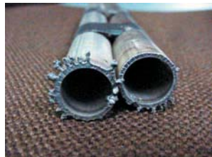
The pressure feed water heaters were tested and found to have severe stress cracks from the back face of the tube sheet in the de-superheating zone extending approximately six feet to the back of the zone
